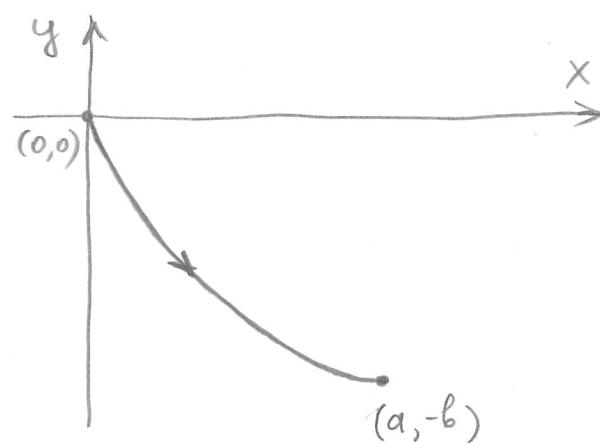
While the straight line connecting the two end points would have the shortest length it is not the path that corresponds to the shortest travel time. This is because the particle (of mass  $m$ ) is accelerated by the gravity force. The lower its vertical position the faster it moves — the kinetic energy is converted from the potential energy.
