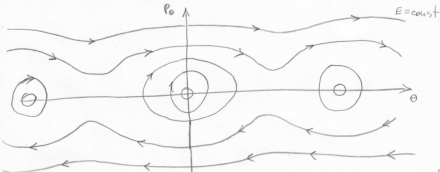
For energies  $E < mgl$  the phase trajectories are closed (ellipse-like) curves. In this case the pendulum oscillates forth and back. For energies  $E > mgl$  the pendulum still has non-zero kinetic energy at the highest point  $\theta = \pm \pi$  and continues its motion without reversal of direction.
