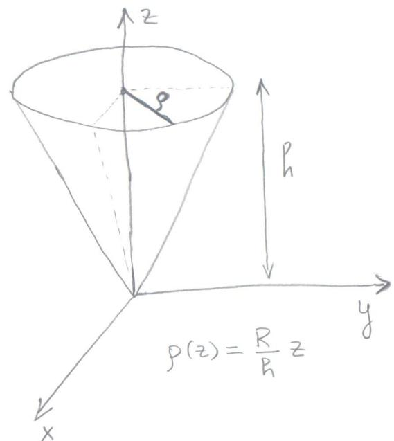
Second, let us find the moment of inertia of the cone about the x-axis (or any other axis lying in the xy-plane)
